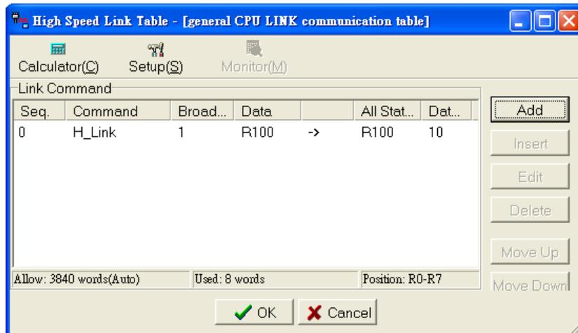
You can also use the “Insert” button to insert a communication command; or select the communication command that you would like to modify, and press the “Edit” button, and you will be able to modify it; press the “Delete” button and you will be able to delete the communication command. Use the “Move Upward” and “Move Downward” buttons to change the order and sequence of the various communication commands.
