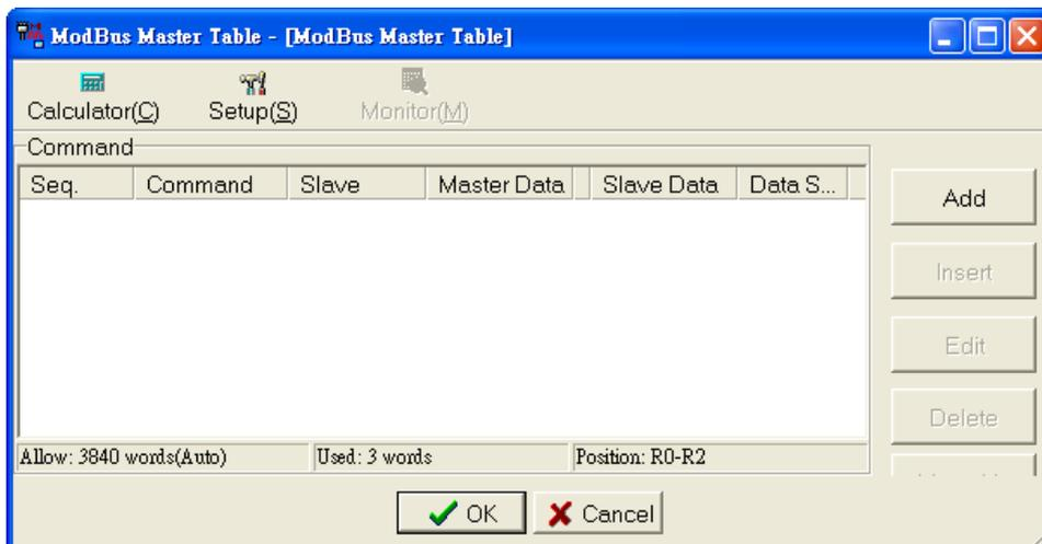
The following procedures are the same as in [Create General CPU LINK Communication Table] in 5.2.1, with features such as “Add”, “Insert”, “Edit”, “Delete”, “Move Up”, “Move Down”, etc. Create three new communication commands, as shown below:
