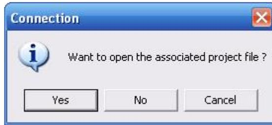
1. Click the "Yes" button: which will open the project file and connect to the PLC. (The contents of this project must be exactly the same as the content of the PLC program to be connected with, or else the connection cannot be made.)
