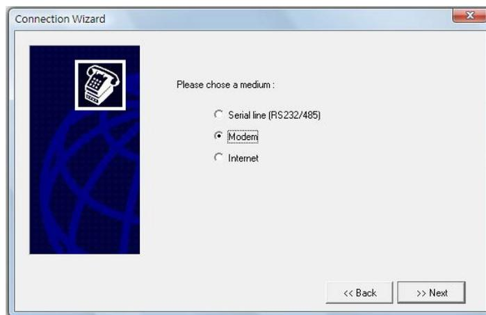
Set the PLC station number and select the modem model, set three dial modes, which are described in the
