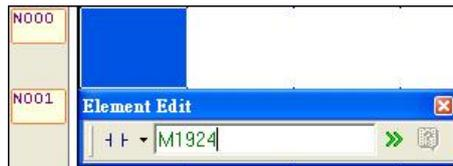
Click on the **F** icon in the component tray, click once behind the "M1924" contact instruction, and then the [Function Lookup] window should appear, select "SFC" under the [Class] option, select "TO" for the [Name], press the "OK" button, and the following window will appear:
