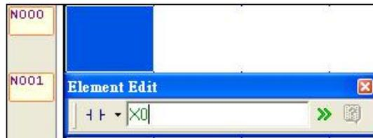
Then you will see a dialog box prompting you to enter the reference number for contact A, enter X0, and now you have completed the input of a contact component in the ladder diagram window:
