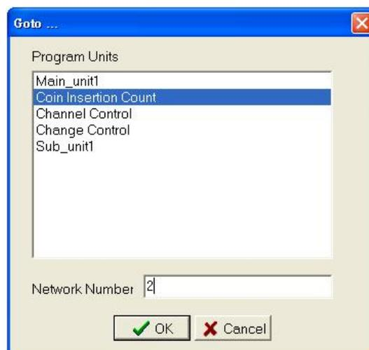
Select "Coin Insertion Count" in the [Program Units], and enter "2" to represent N002 in the [Network Number]. Press "Confirm" button, and the cursor will move to the position of the network you are looking for:
