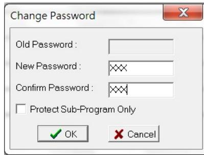
After you have entered the password, all subsequent access to the project will require inputting this password to protect the program.
