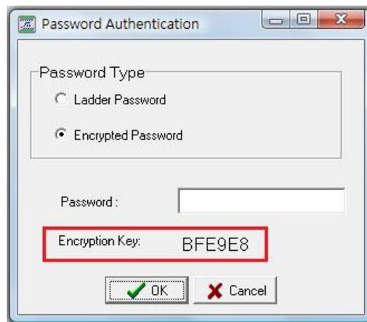
If an encryption password is used, then the user that wishes to perform the recovery must give the encryption key shown in the window to a protector who knows the program password. The protector have to open a new WinProladder, then executes [Tools] → [Encrypted Password Generation] :
