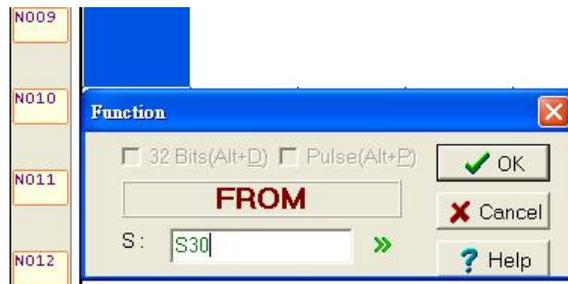
Enter “S30”, press “OK”, and the FROM function will appear. Use the cursor to select the contact A and single-click the point right behind it, enter the reference number “X3”; or directly enter “AX3” behind it, as shown in the following window:
